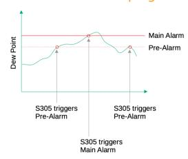
Two alarm levels can be programmed (pre and main alarm), serving an optical indications or separate relay outputs.
