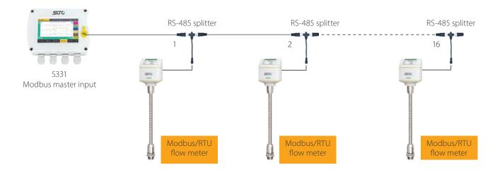
Flow meters can be easily integrated into a Modbus/RTU network (daisy chain)
