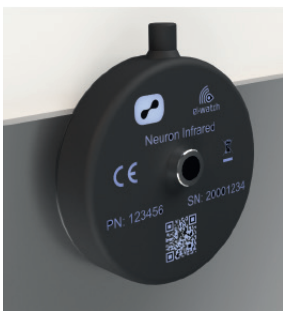
Place elevated with distance to fixed objects
