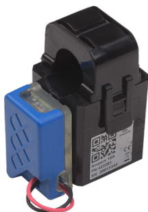
Neuron Ampere sensor for compressor energy consumption monitoring
