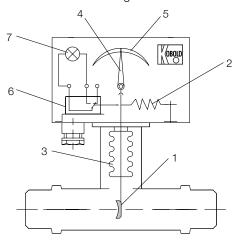
The motion is transferred positively from the baffle (1) to the measuring section.
