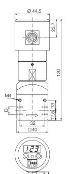
DPM-...L with analogue output and plug-on display DPM-...Z with analogue output and pointer indication
