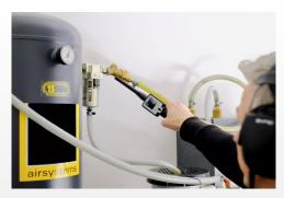
Leak detection with focus tube
